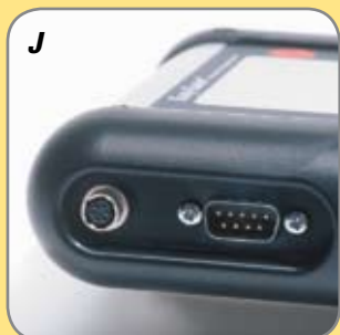
Countersunk connectors, well protected against external damage.
